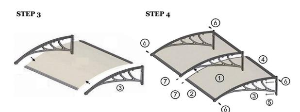
Mount the assemble board on the brackets and connect them with bolt G and O. (It's recommend to place the board vertically
