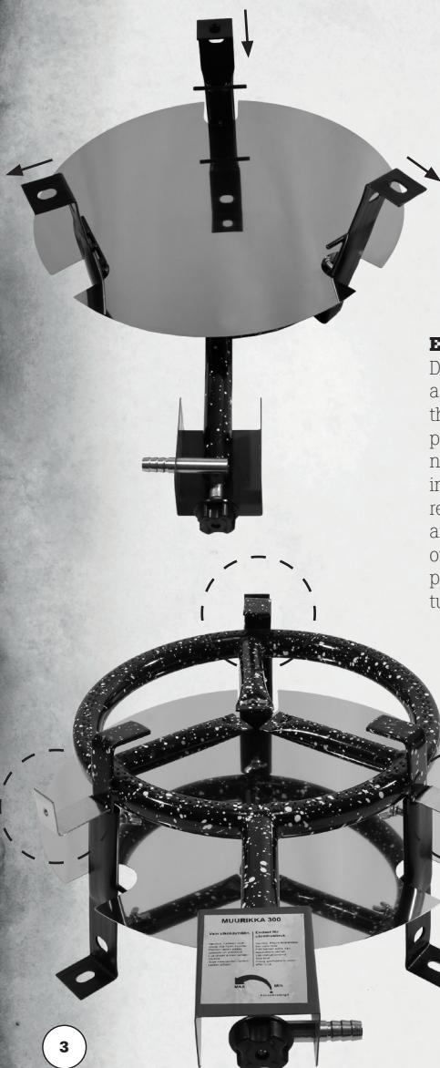
**ENG** Place the gas burner ring D-300 upside down on the assembling surface. Fasten the short legs with the heat protective plate to the gas burner ring's short legs as shown in the picture. Note that the rear leg's bending is inwards and the front legs' bending is outwards. The heat protective plate's support pegs should be turned inwards.
