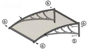
Drill four holes before installing the canopy. Make sure the holes you drill can exactly match to the holes of the bracket.
