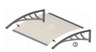
Mount the assemble board on the brackets and connect them with bolt 6 and 7. (It's recommend to place the board vertically when mounting the brackets.)
