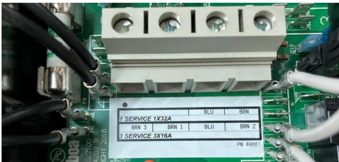
We need to follow the instructions of "3 SERVICE 3X16A", the first interface is connected to the fire wire (BRN 3), the second interface is connected to the fire wire (BRN 1), the third interface is
