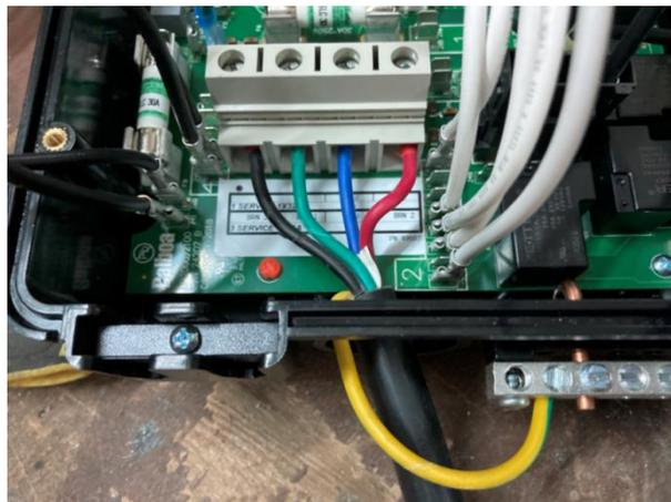
**Important!** A leakage protection switch with a current not less than 20A and a leakage current no more than 30MA should be installed in current front-end.
