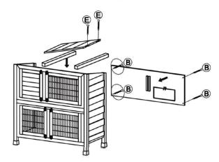
3. Secure the back panel(top) to the left and right panels with 4 xB screws.Place the wooden strips to fix the ladder location.Fix the ladder with 2 xE screws.
