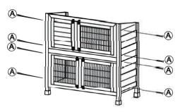
1. Attach the front panels(top and bottom) to the left and right panels using 8 xA screws.
