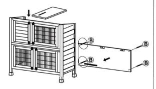
Secure the back panel(bottom) to the left and right panels with 4 xB screws. Place the floor (on the left side).
