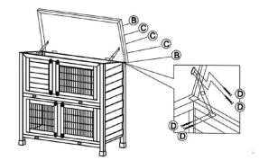
5. Attach the roof to the back panel(top) using 2 xB and 3 xC screws. Fix the hinges to the left and right panels and the little piece of wood on the underside of the roof.
