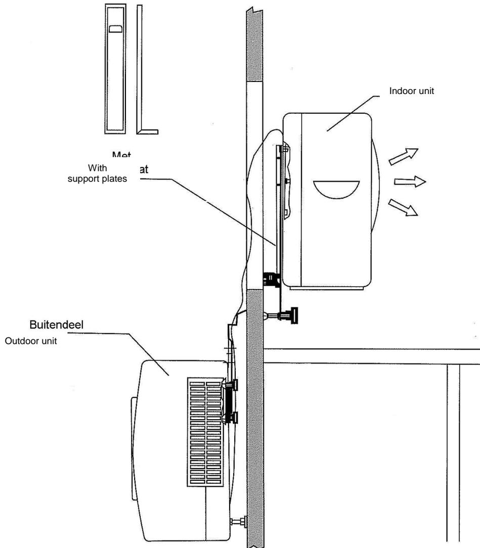
At the indoor side, attach the support plates to the brackets using the female-threaded knobs. Now you can slide the indoor unit over the support plates.
