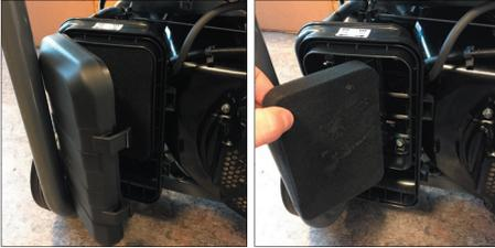
Clean the filter element in hot water and mild detergent. Rinse with clean water. Press the water out of the filter element and allow it to dry. Pour new engine oil onto the filter element, and press any excess oil from it. Replace the filter element, and replace the cover.
