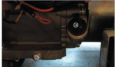
Open the oil bung (14) and unscrew the oil drainage cap. Tilt the generator and drain the used engine oil. Dispose of the used oil in accordance with local rules and regulations.
